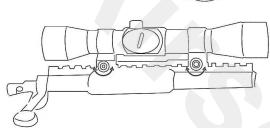
• Engage the sight by turning the switch. Turning the switch at 3 position will open the sight with the hightest light (GS13 only), turning the switch at 2 position will open the sight with highter light, turning the switch at 1 position will open the sight with dark. Turning the switch at 0 position will close the power.
