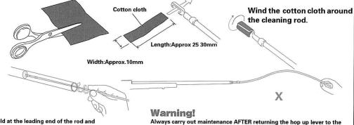
Hold at the leading end of the rod and insert the rod into the barrel while turning the rod.
